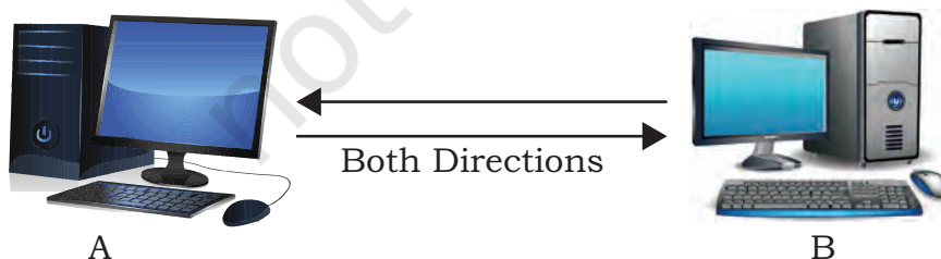
Figure 11.5: Full duplex transmission of data
